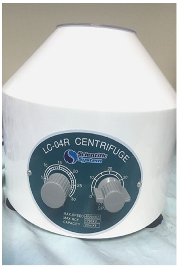
Fig. 1 The tube is placed in the centrifuge at 3500 rpm for 20 min
